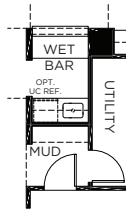
OPT. WET BAR ILO STORAGE 2 CANNOT BE SELECTED WITH OPT. LEARNING CENTER
